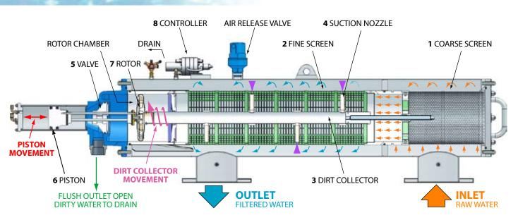
During normal filtering mode the raw water enters the Inlet of the filter, passes through the Coarse Screen (1), (the 7 mm perforations remove large debris that may obstruct the lower mechanism). Water then travels to the inside and through the Fine Screen (2) to the Outlet.
